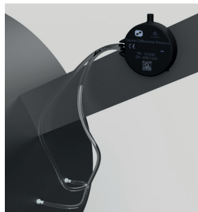
Keep antenna clear off the metallic surface
